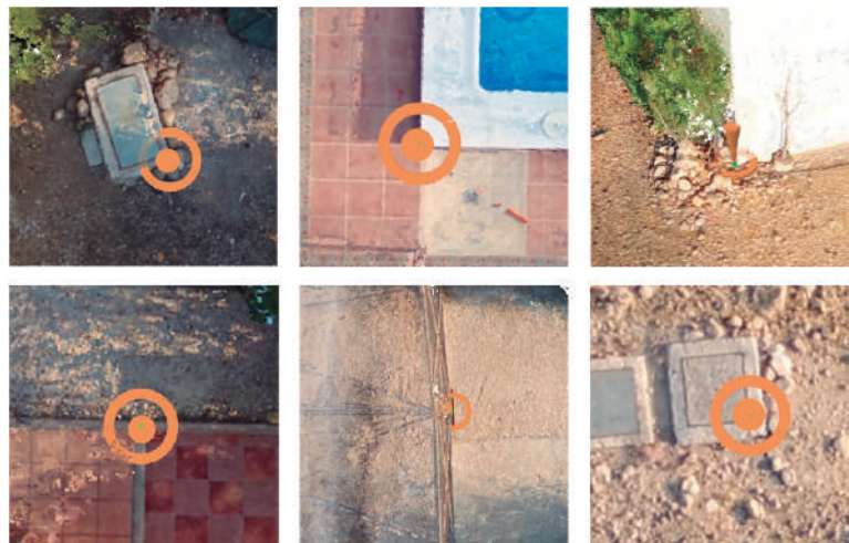
Figure 4. Meaningful objects used as marks for an accurate georeferencing.
