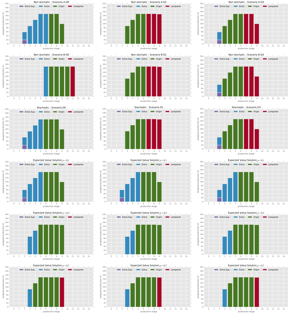
Figure 5: Production plans for the scenarios considered in Section 3.3. Columns correspond to the three different quality evolution scenarios. First and second row show the optimal production plans supposing perfect information for price Scenario A and B, respectively. Third row represents the recourse problem solution. Rows 4 to 6 represent the expected value solution to the problem for p = 0.1 , p = 0.3 and p = 0.7 , respectively
