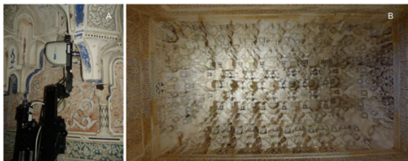
Figure 1. In situ measurements in the Hall of the Kings: detail of the probe head attached to the videomicroscope (A) and panoramic view of one of the small rectangular vaults (B).
