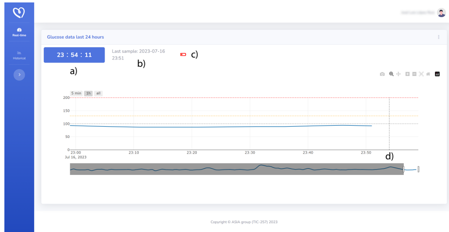
Fig. 5: Web application interface for the first type of monitoring: a) Current time, b) Time instant when the last sample was received, c) Remaining smartphone battery and d) Vertical bar showing the current minute (own image).
