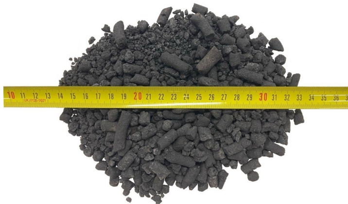
Figure 10: Charcoal from gasification of exhausted olive pomace pellets in a downdraft gasifier.
