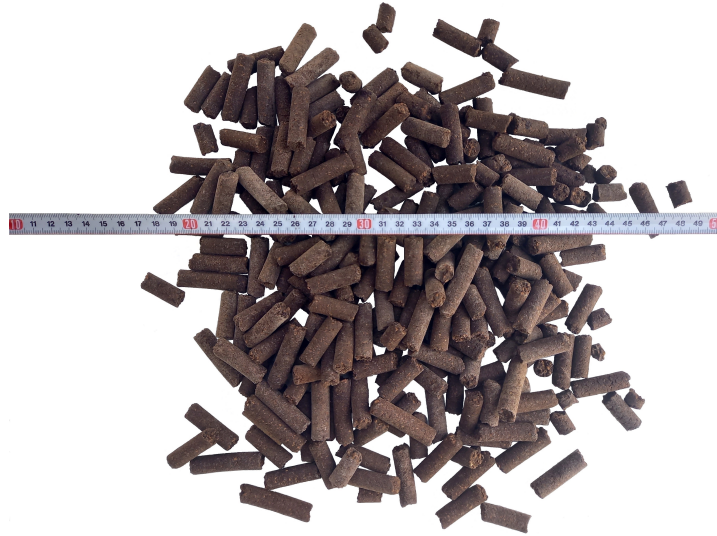
Figure 1: Exhausted olive pomace pellets used as feedstock for the gasification plant.
