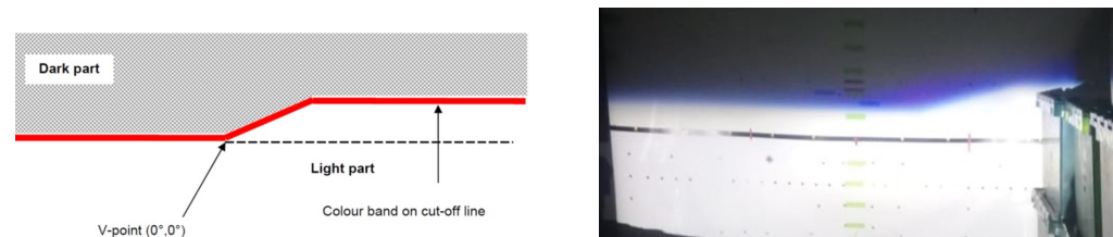
Figure 1. The low-beam lighting pattern. Left: the cut-off line shape; right: low-beam projection in an inspection tunnel.
