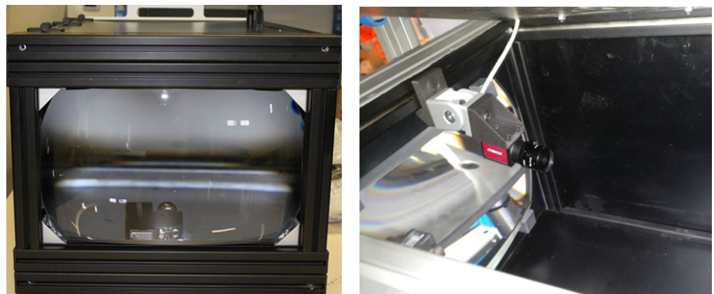
Figure 6. Image acquisition devices. The photometric tunnel and the colour camera inside the tunnel.
