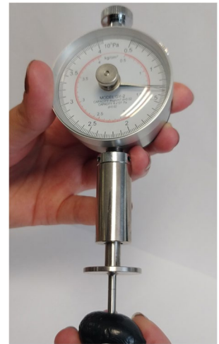
Fig. 1 The measurement process with the penetrometer device
