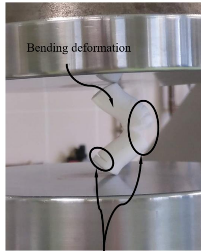
Layers delamination and fracture of the filament
