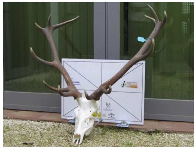
Fig. 8 – Metric reference element of known dimensions behind the antler (rectangular plate of 594 \times 420 mm).
