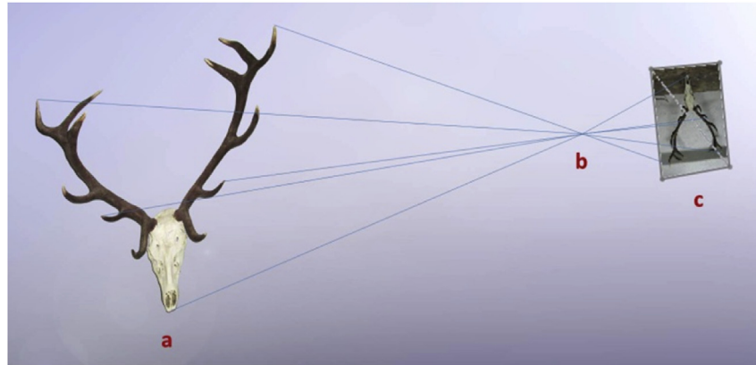
Fig. 5 – Trajectory of the rays of incidence on the plane of a photograph. a) Real object; b) position of the camera lens; and c) photograph (reduced in scale and inverted).
