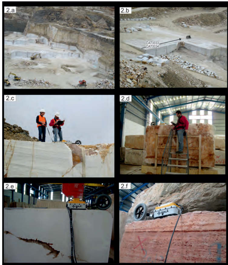
Figure 2: Photographic prints. General view of the Macael quarry under study (2a). Location of the profiles of Fig. 3 (2b). Details of the data collection using the 250 MHz antenna (2c). Study of blocks prior to the rolling process (2d). Study of a block of Crema Marfil with visible cavities; its GPR response is used for comparison purposes (2e). Study of a block of Red Travertino using the GPR technique; an evident horizontal layering is observed (2f).
