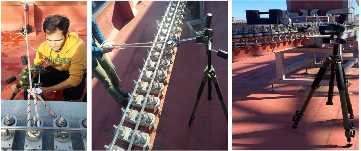
Figure 15. Measurement of track response to concentrated loads. Lateral loading with pulley, mass and dial gauge (left), lateral loading with dynamometer and dial gauge (center), and vertical loading with mass and dial gauge (right).
