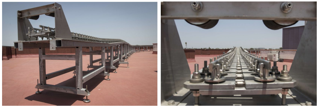
Figure 13. Structure with ascending and descending slopes (left) and buffer stops at the end of the track (right). Photographer: Ludivine Mimar.
