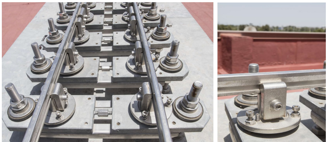
Figure 12. Support mechanisms (left) and rail to support mechanism clamp (right). Photographer: Ludivine Mimar.
