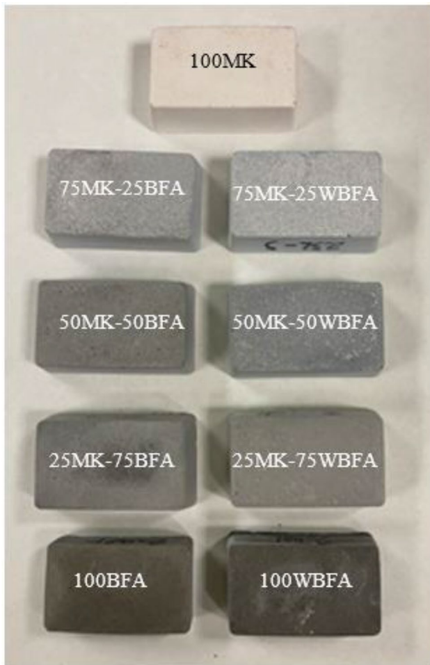
Fig. 6 Alkali-activated bricks prepared as described in experimental procedure
